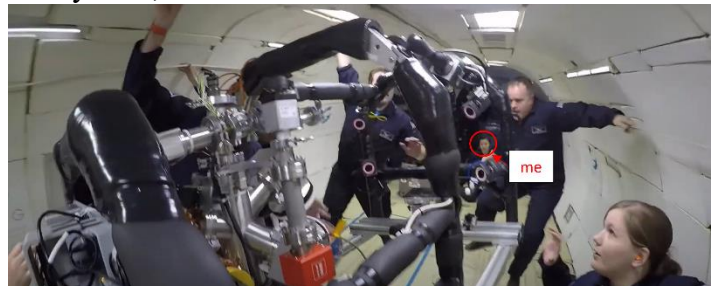
Figure 2: microgravity flight experiment characterizing docking technology performance
